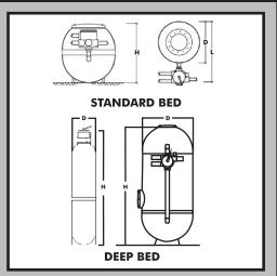
The DAYLIFF 'CX' filter range of industrial specification filters have been specially developed for institutional and commercial applications where higher levels of operating performance and reliability are demanded. Their design combines leading filter technology with many years of GRP production experience and the result is a range of quality products suitable for both swimming pools and general water treatment uses. Features include:-
