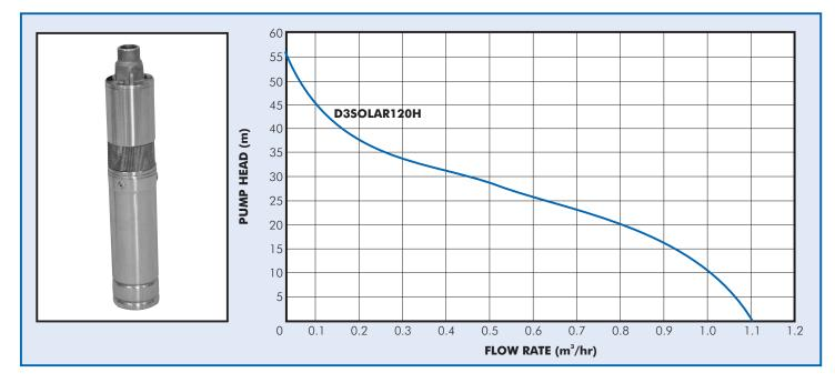
The DAYLIFF D3SOLAR pump is specifically designed for PV solar powered water supply from wells and boreholes.
