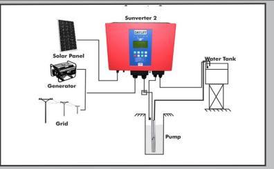
Dayliff Sunverter 2 is an advanced AC/DC inverter specially designed for solar powering AC motors in various water pumping applications. A particular feature is hybrid capability that enables for the connection of direct AC power from mains or generator supply. It is adaptable to all AC motor types and can be retro fitted to the solarisation of existing AC supply installations. Particular features include;
