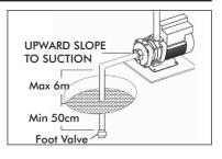
If the suction depth exceeds 4 meters then a one size larger diameter pipe should be used, though for maximum pump performance suction height should be minimised.
