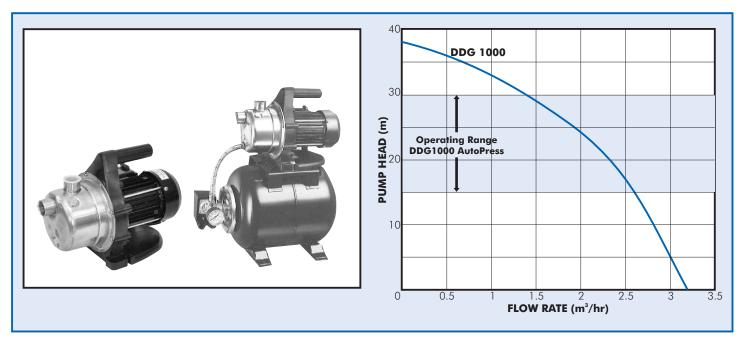
The DAYLIFF DDG pump is of single stage centrifugal impeller self priming design suitable for small scale irrigation, water boosting and water transfer applications. Also available is the 'AutoPress' booster system which incorporates a 19L horizontal diaphragm tank, pressure switch and pressure gauge for automatic pump operation.
