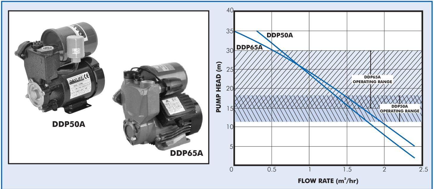
The DAYLIFF DDP50/65A are compact and efficient automatic pressure controlled peripheral impeller booster pumps suitable for domestic and small scale applications where on-demand water supply is required.
