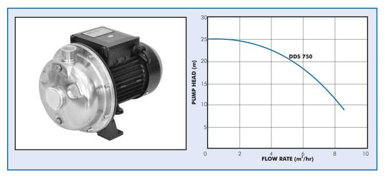
The Dayliff DDS pump is of centrifugal single impeller non-self priming design suitable for water supply, agriculture and industrial applications for slightly corrosive liquids or where high levels of liquid purity is required.
