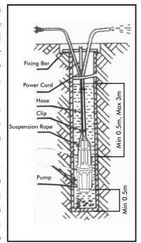
• Once installed it is recommended that the suspension rope, drop cable and outlet hose be tied together with cable clips or tape at approx 1m spacings with the first tie approx 200mm above the pump.
