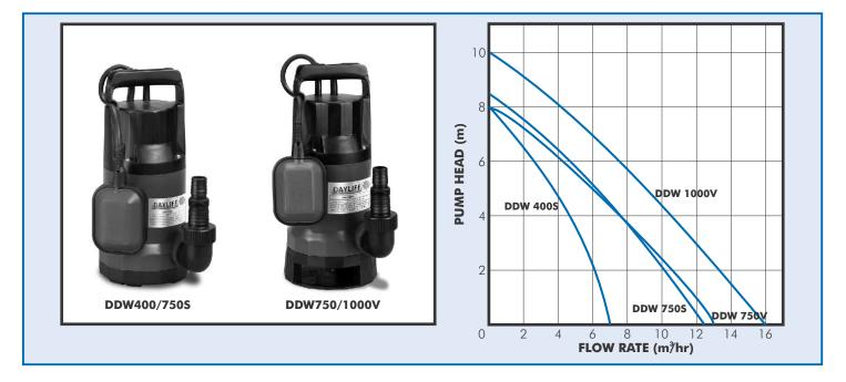
The DAYLIFF DDW submersible pump range are centrifugal submersible pumps designed for small scale drainage, irrigation, fountain and water transfer applications. Two versions are available, the standard S version with open impeller for lightly turbid water and the vortex V version for water with higher silt loads.
