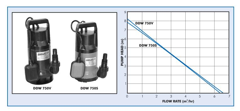
The DAYLIFF DDW submersible pump range are centrifugal submersible pumps designed for small scale drainage, irrigation, fountain and water transfer applications. Two versions are available, the standard S version with open impeller for lightly turbid water and the vortex V version for water with higher silt loads.
