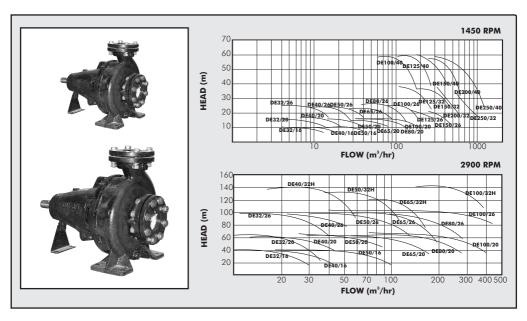
The **Dayliff DE** range of end suction centrifugal pumps are rugged heavyduty pumps designed for various water supply, irrigation and fire fighting duties in agricultural, commercial and industrial applications. The pumps feature gland packing seal for simple and economic maintenance, back pullout design enabling removal of the rotating element without disturbing the pipework connections and heavy duty bearings.
