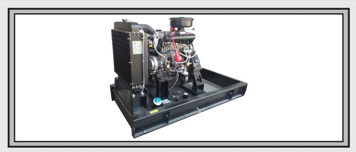
Dayliff DLY prime mover diesel engines are of 4-stroke, direct injection, water cooled design suitable for a wide range of stationary industrial and agricultural applications including water pumps, firesets and generators. All models are naturally aspirated cooled by forced water circulation and settable for fixed speeds between 1500 to 3000rpm.
