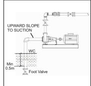
**Pipe Supports:** Piping should be supported independently near the pump. Pipe loads on the pump flanges must be avoided.
