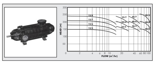
The DAYLIFF DMS range of horizontal multistage centrifugal pumps are heavy duty industrial quality pumps suitable for various water supply, irrigation and industrial applications. Particular features include gland packing seals for simple and economical maintenance and external securing tie bolts for ease of disassembly. Construction is heavy duty cast iron stages and pump body, with cast iron impellers and diffusers and stainless steel shaft.
