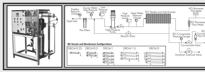
Reverse Osmosis is a proven technology to remove dissolved solids in water. At the heart of the system is the membrane, though the effectiveness of treatment relies on the correct matching of all components to provide an efficient treatment process, DAYLIFF plants being carefully engineered to provide reliability with the highest treated water quality.
