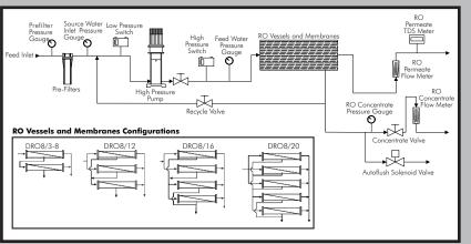
Reverse Osmosis is a proven technology to remove dissolved solids in water. At the heart of the system is the membrane, though the effectiveness of treatment relies on the correct matching of all components to provide an efficient treatment process, DAYLIFF plants being carefully engineered to provide reliability with the highest treated water quality.
