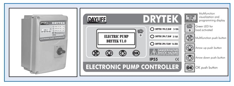
The Dayliff Drytek Electronic Pump Controller is a solid state integrated control unit for all types of pumps with a particular application to borehole installations. Panels are fitted with a digital display of both operating and fault parameters and settings are simply made using fascia mounted push buttons. A range of sizes are available for single and three phase motors, settings for particular motor sizes being effected by simple adjustment of the running current.
