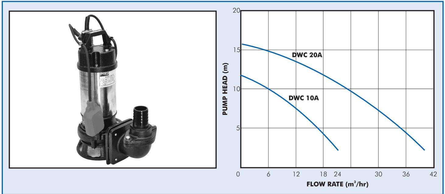
The Dayliff DWC range of heavy duty submersible pumps are designed to handle industrial and domestic waste water and sewage with a specially designed cutter impeller. They are suitable for pumping water containing a high proportion of solid particles including threads and fibres.
