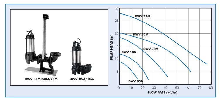
The Dayliff DWV range of vortex impellers submersible pumps are designed to handle industrial and domestic waste water and sewage and are especially suitable for pumping water containing a high proportion of solid particles.
