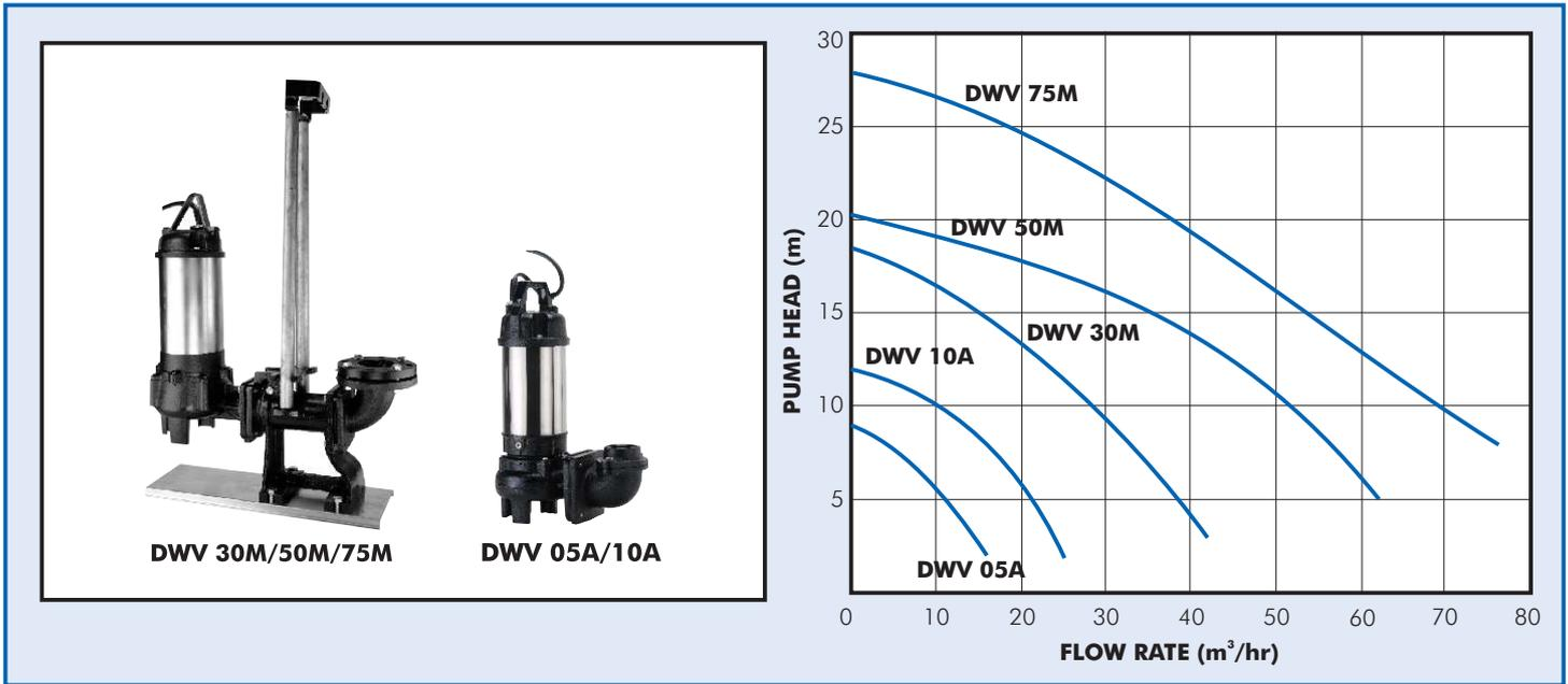
The Dayliff DWV range of vortex impellers submersible pumps are designed to handle industrial and domestic waste water and sewage and are especially suitable for pumping water containing a high proportion of solid particles.
