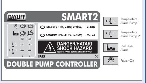
The Dayliff Smart 2 is an integrated electronic controller available in single and three phase for the automatic operation of two pump installations with special application to automatic booster sets. It includes an electronic circuit board that provides the control functionality as well as standard incoming power and pump operating auxiliaries mounted in an ABS enclosure to give a complete control solution.
