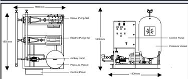
DAYLIFF FLA packaged Fire Sets are specially designed to provide automatic supply to multiple hose reel or sprinkler outlets for firefighting installations. Standard sets combine parallel duty diesel and electric powered supply pumps to ensure serviceability in all conditions as well as a jockey pump to maintain system pressure. Particular features include:-
