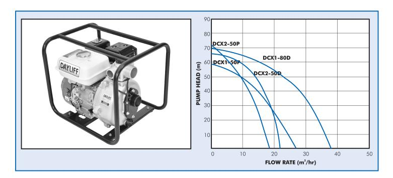
The DAYLIFF DCX range of portable high pressure engine are of self priming closed impeller centrifugal type suitable for high head water transfer, irrigation and fire fighting applications.
