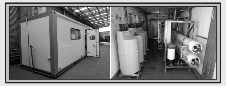
With production capacities up to 100,000 lit per day, the Dayliff Mobile Water Treatment Plants are designed to be deployed quickly wherever temporary or emergency potable water is needed and accommodate a wide variety of feed sources including saline, turbid or highly mineralized water.
