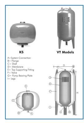
Pressure tanks are important components of pressurised booster supply systems where automatic pumped water supply is provided by means of pressure switch controlled pumps. The tanks have two functions; to cushion pressure surges as the pump starts and stops and also to provide a drainage supply into the system to control pump cycling.
