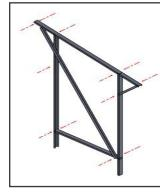
Assemble the individual support structure sections as per the drawing. The sections are delivered in pieces according to the structure design with the members loose. Secure all joints firmly on both sides with the self-drilling screws provided using an electric drill with appropriate screw bit.
