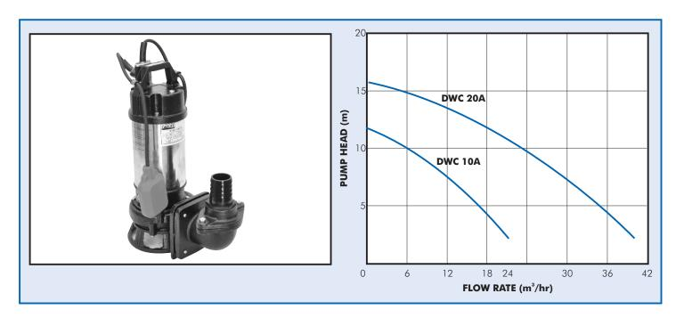
The Dayliff DWC range of heavy duty submersible pumps are designed to handle industrial and domestic waste water and sewage with a specially designed cutter impeller. They are suitable for pumping water containing a high proportion of solid particles including threads and fibres.
