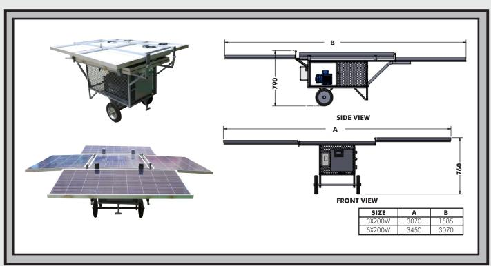
Daily SunBarrow is an innovative accessory for small scale solar PV applications were mobility and security are important requirements. The unit includes a wheel mounted enclosure where batteries and accessories can be stored topped with a hinged platform that opens out for PV module mounting.
