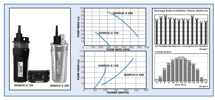
DAYLIFF SUNFLO-S series submersible pumps are designed for reliable small-scale water supply from boreholes and wells and are the ideal solution for remote pumping requirements in livestock watering, irrigation and general water supply applications. They are of positive displacement three-chamber diaphragm design and can run dry without damage. An internal bypass is also incorporated to prevent pump damage in the event of delivery cut-off.
