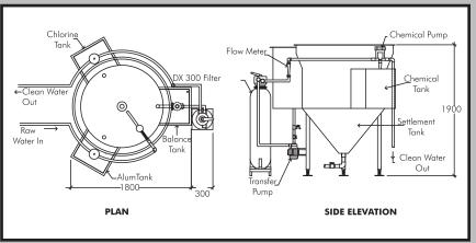
The DAYLIFF 'WG' Water Purifier is an integrated water treatment plant specifically designed to treat the majority of surface waters including the removal of silt, suspended solids and bacteria in small-scale domestic, institutional and commercial applications. The units are simple to operate, low cost and easy to maintain and can provide consistent water quality to WHO standards. Features include:-
